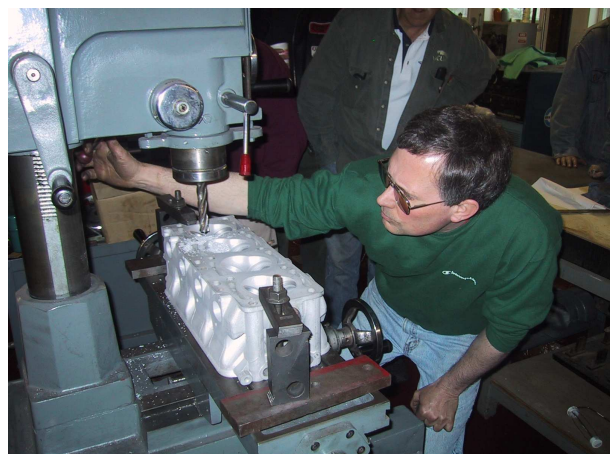
Steve Dutcher repairing a cracked aluminum cylinder head
