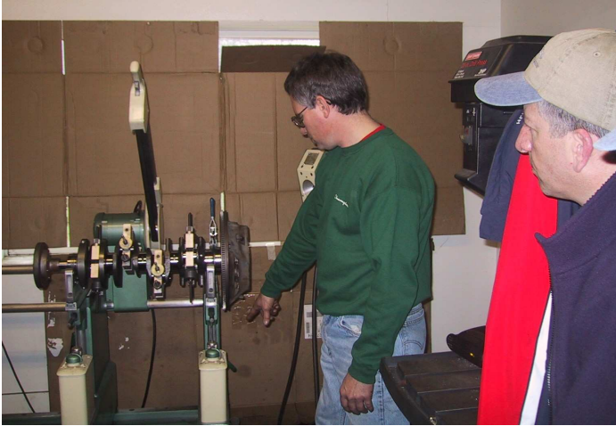
Steve Dutcher demonstrating the engine balancer
